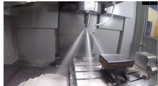
"Our aim is to increase the period between tip regrinds, this is one of the major requests from our customers" explains Pearce. "We now have tools out on test that have directional apertures, which are aimed exactly at the area where the tip contacts the part. The team here are really excited about the potential this gives us. We can print any aperture we need and route the coolant pathways anywhere through the body".
