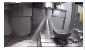
"Our aim is to increase the period between tip regrinds, this is one of the major requests from our customers" explains Pearce. "We now have tools out on test that have directional apertures, which are aimed exactly at the area where the tip contacts the part. The team here are really excited about the potential this gives us. We can print any aperture we need and route the coolant pathways anywhere through the body".
