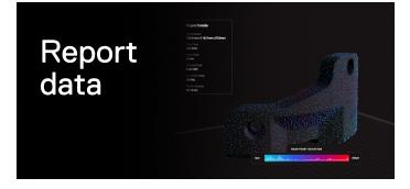
View the deviation across the part's geometry, and set tolerance limits to assess part quality. The print report is saved in Eiger and can be referenced at any future date.
