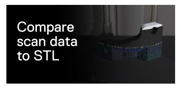
Blacksmith collects measurement data during the print, and assembles a point cloud for review in Eiger. This point cloud is automatically registered and overlaid on the input STL for comparison.
