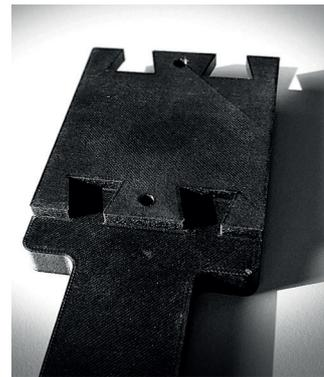
„We have developed a welding machine for foam profiles. We printed all the dies needed for these profiles. Conventional production would have been far more expensive.“ Even a mould to coat parts of an extraction unit with synthetic resin was printed completely. In addition, various other highly complex components of a sophisticated machine extraction system are manufactured with HSHT glass fibre reinforcement.
