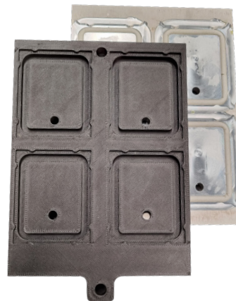
Vacuum Part Holding Jig printed on FX20.
