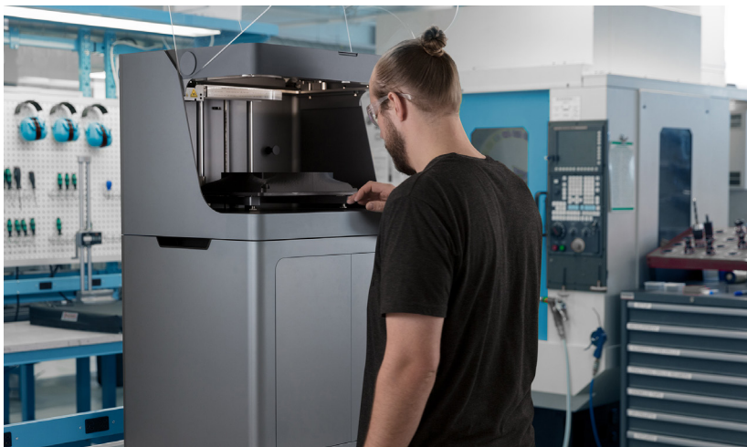
2. 3D printers can complement the machine shop by producing complex, high-strength manufacturing tools and fixtures.
